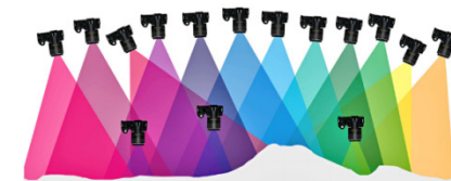
FIGURE 8-14 Acquire photos converging on a feature, at multiple distances and angles. From Shervais (2016, Figure 12).
