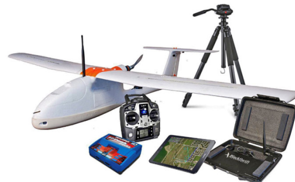
FIGURE 8-15 Components for operating a sUAS. Courtesy Black Swift Technologies.
